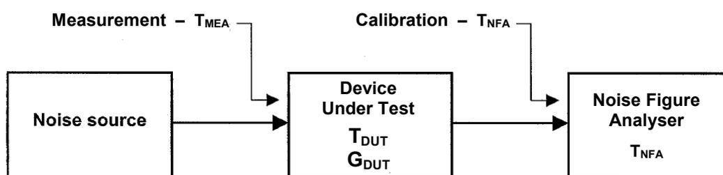
Figure 1: Test setup for Y-factor noise measurements
