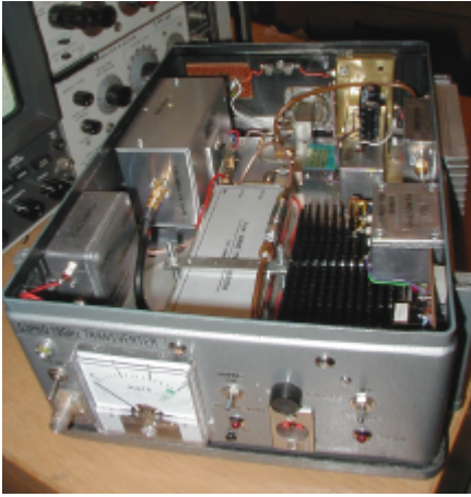
A 10GHz narrowband system based around a DB6NT basic transverter kit, a GBACE designed ovened crystal oscillator kit and a DB6NT ready made 5W PA
