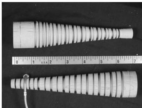
I repeated with a 0.086 diameter drill bit for UT-085, placing these grooves between the others.
