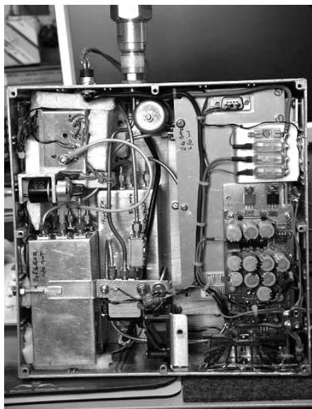
The photo above shows G4ALY's latest home-brew transverter for 3.4GHz. It's based around a surplus Ionica receiver module and a 15 watt Ionica PA. Please look for Ralph on the band during the contests this season. He's in IO70VL.
