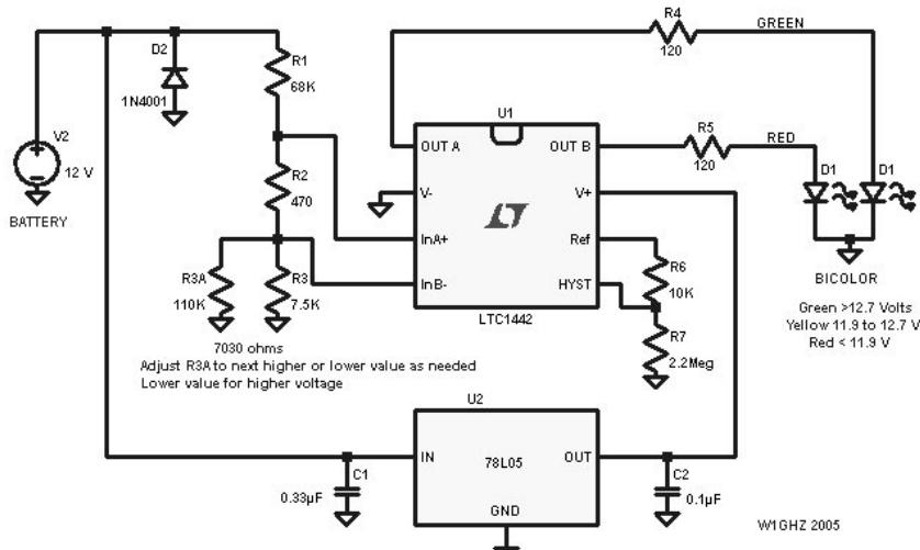
tween the on and off trip points. The LTC1441 has a pin for adding hysteresis, by adding R6 and R7. The values shown provide about 0.1 volts difference between the on and off voltages.
