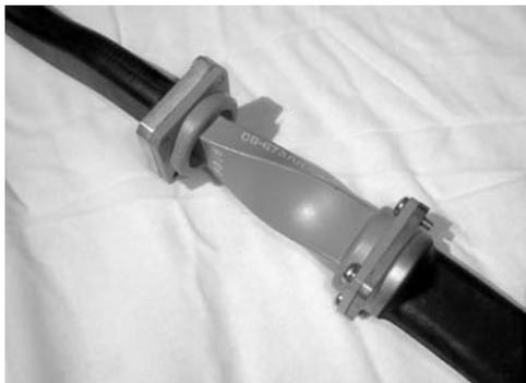
Getting waveguide to go around a rotator, or even to be flexible going up a portable mast, can be fun. Waveguide has E and H planes. One way to remember which is which, is it to think of these planes as Hard and Easy to bend.
