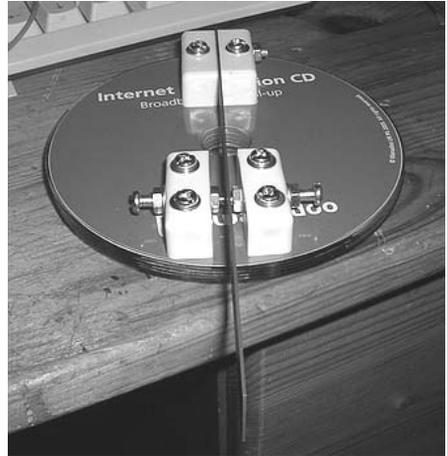
Above is a photo of the completed paddle key, which consists of 6 Wanadoo CDs glued together, 4 plastic shelf supports and several nuts and bolts. I used a spring steel ruler for the paddle.
