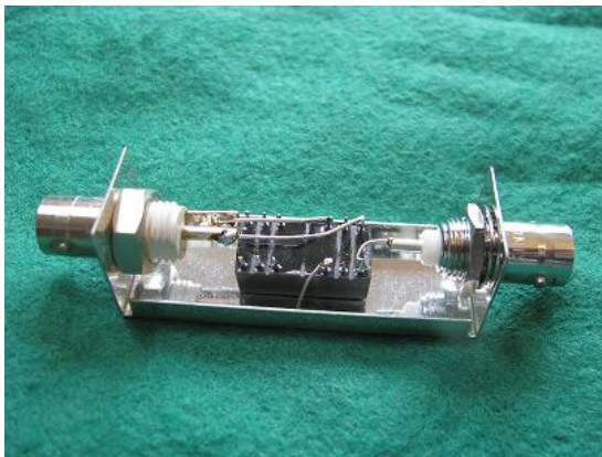
Fig 5 – A recovered filter assembled in a small tin-plate enclosure, with insulated output connector
