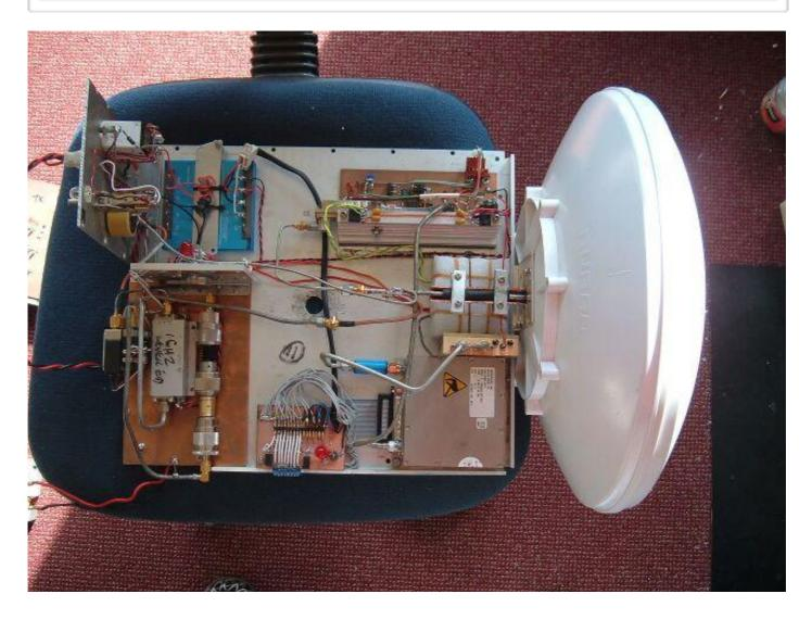
After reading an Article (1) written by Kerry Banke – N6IZW, I became enthused with building gear for 47 GHz. It was not long however before I realised I had all the parts needed to build a 76/78GHz transverter instead. This home-brew, prototype transverter is with just one exception - ALL coaxial.
