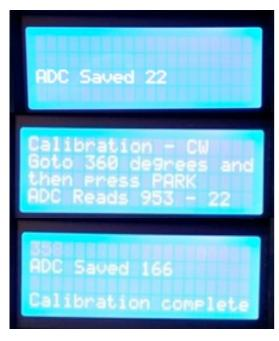
Pressing the PARK button saves this ADC value in EEPROM (MINOffset) which is then subtracted from ADC reads in the main code.
