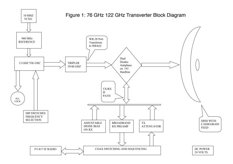
(surplus 14GHz mixers) mounted/soldered on the end of a piece of .141 hardline. A photo of some prototype mixers can be found later in this document. A small flared horn is fitted over these diodes and this "feed" is then slide through a rear dish mount and aimed at an integrated Cassegrain reflector in the radome of a 300mm dish. The positioning of this horn relative to the diodes is VERY critical. Correctly positioned, a performance improvement of more than 15-20dB
