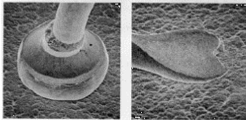
After the first bond is made to the die then the wire is pulled through the bonding tool and then pressed onto the track/frame and ultrasonic energy used to make the weld. Ball bonding isn't used much with microwave devices.
