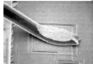
Heat is provided to the die/assembly on unit known as a work stage. Typically this is heated to 125C. Some processes call for the tool to be also heated in place of, or in combination with, the ultrasonic burst. Every MMIC manufacturer seems to have slightly different bonding parameters.
