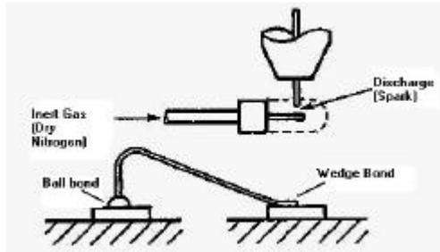
Ball bonding relies upon creating a blob of molten metal just a fraction of a second before the wire makes contact with the pre-heated die/track/package frame and then it is pressed down. Why pre-heated? If you think about it, putting a hot blob against a cold piece of metal isn't going to give an alloyed joint. This method of bonding is ideal for some devices and probably a large proportion
