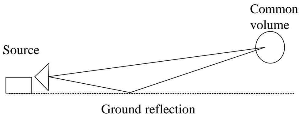
Figure 1 shows the ground reflection range with the source antenna close to the ground and the common volume in which the measurements are taken.
