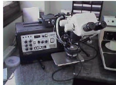
The trickiest bits are getting the force right and applying the energy. The first is solved with some simple mechanics and in modern machines, strain gauges. And with the second there are two main methods of bonding – thermosonic/ball bonding and thermocompression bonding.
